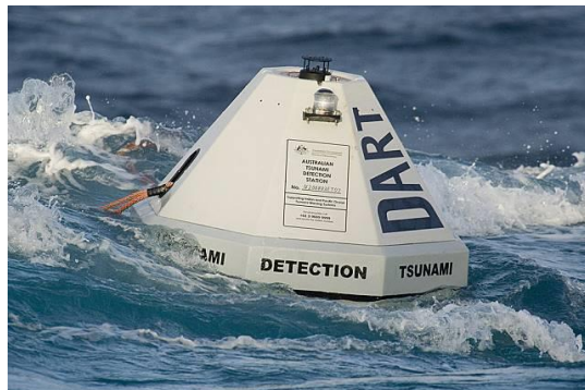
Gambar Pelampung khusus ( Deep Ocean Assessment and Reporting of Tsunamis )
